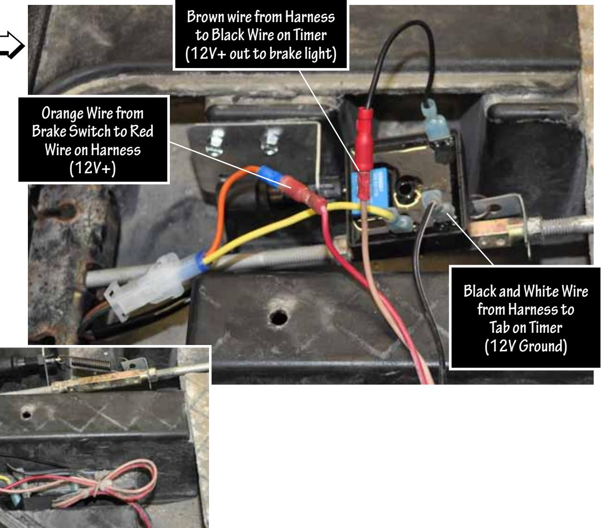
13. With key switch ON, depress and lock parking brake to test brake lights. If they do not light, adjust switch, disconnect connector to brake light switch and turn adjusting nut on brake light switch for proper tension on spring.
