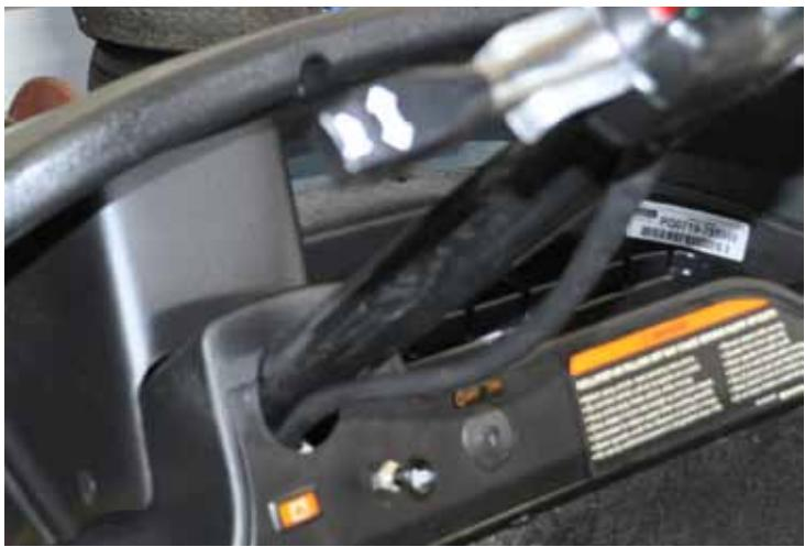
19. Fit harness assembly in dash. Route Signal indicator Harness through round opening with steering column. Attach dash panel with screws retained in step 1.
