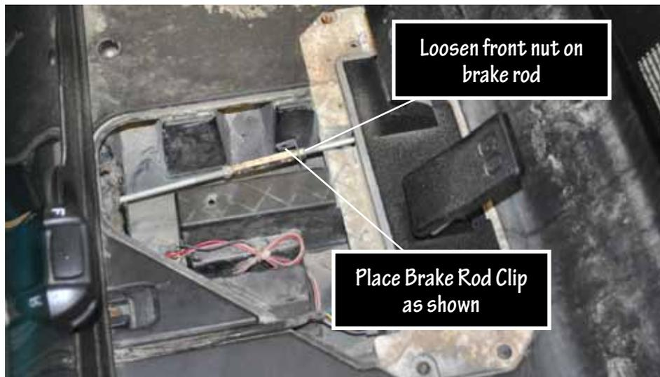
Loosen front nut on brake rod
