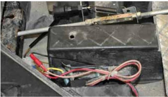
13. With key switch ON, depress and lock parking brake to test brake lights. If they do not light, adjust switch, disconnect connector to brake light switch and turn adjusting nut on brake light switch for proper tension on spring.
