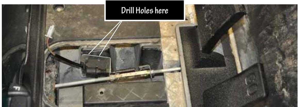
10. Bolt Brake Switch Bracket to Frame.
