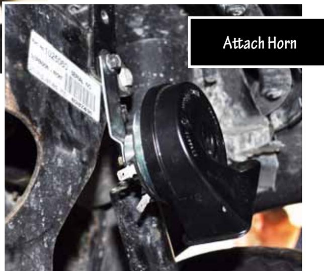
17. Attach black and orange wires on Headlight assembly to Horn.
