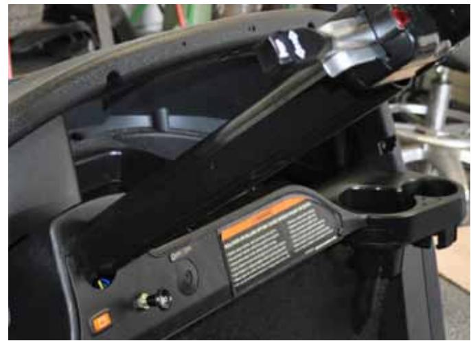
20. Snap on Steering Column Cover. Gutter of Cover is for Signal Indicator Harness.
