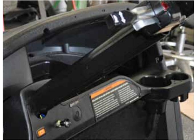
20. Snap on Steering Column Cover. Gutter of Cover is for Signal Indicator Harness.
