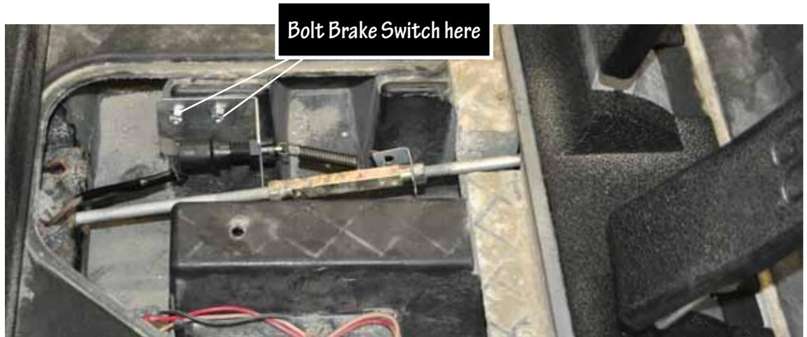
11. Plug timer relay into brake switch.
