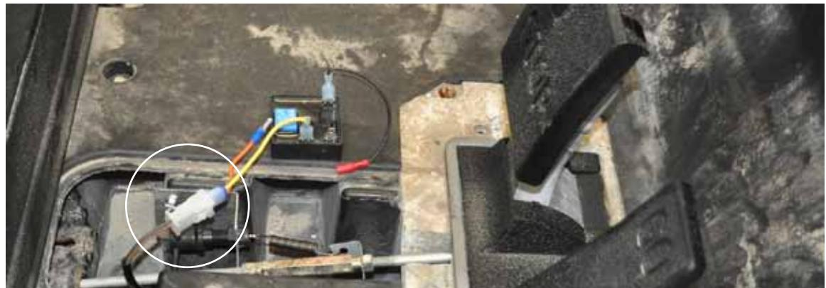
12. Pull out existing harness. Connect wires as instructed in photo. Place brake light assembly in right side of well as shown.
