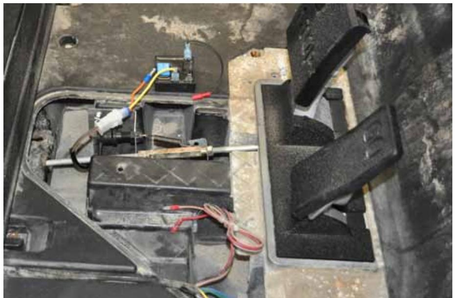
16. Install Horn. Remove Headlight by removing bolts that secure light to vehicle frame. Retain hardware. Remove and retain bolt from support bracket under front end of vehicle on the driver side near VIN tag. Use bolt to attach Horn.
