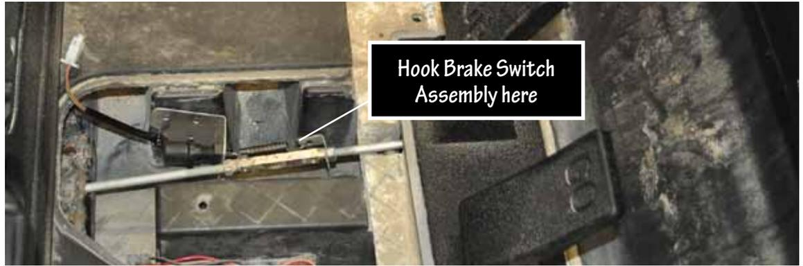
9. With Parking Brake OFF, put slight tension on spring of Brake Switch. Use Bracket as template and drill two 1/8" pilot holes.
