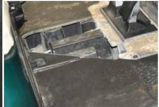
6. Remove Floor Mat and brake cover plate.
