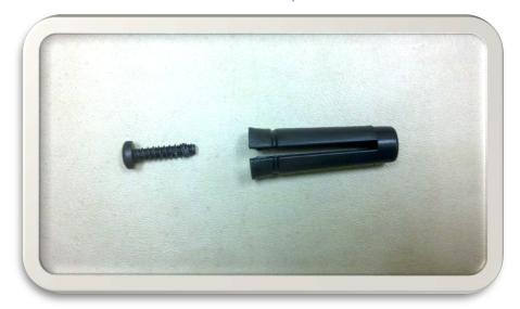
5) After removing screw from original dash, install dash peg holder (above) by re-using original screw. The dash peg will be held on the dash by peg holder and O-ring. Screw peg holder onto the golf cart.
