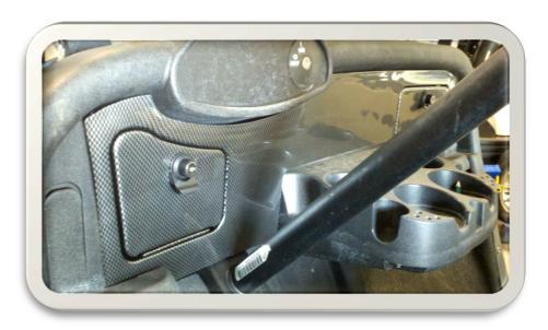
6) Snap dash into each peg holder by lining up the pegs sticking out of the replacement dash and snapping into place.
