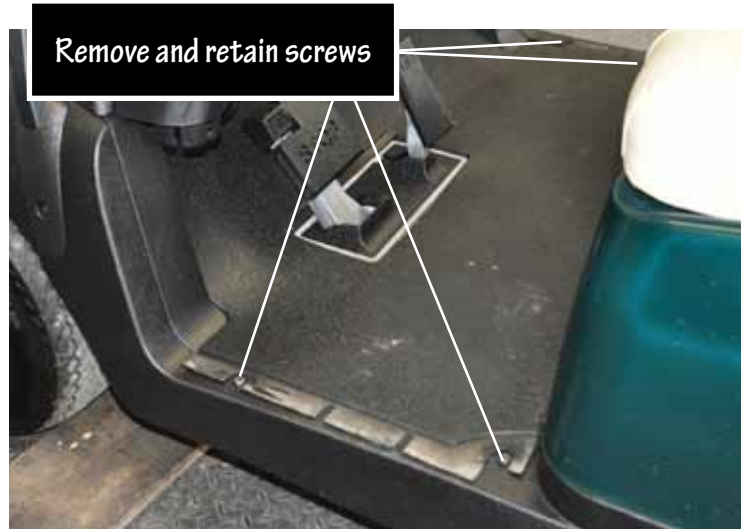
5. Remove and retain 4 torx head screws from floor panel of vehicle.
