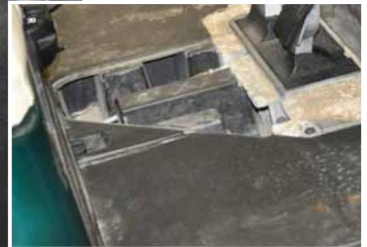
6. Remove Floor Mat and brake cover plate.
