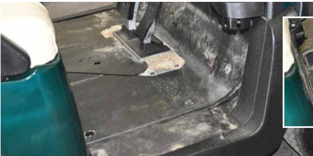
6. Remove Floor Mat and brake cover plate.
