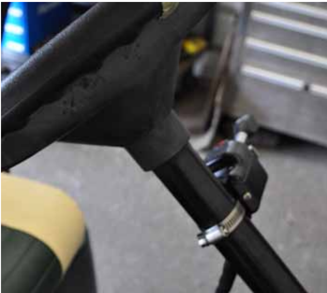
4. Attach turn signal indicator to steering column with Hose Clamp.
