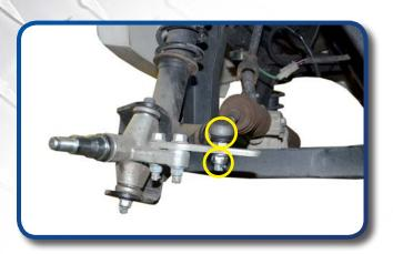
Disconnet ball joint by removing cotter pin and castle nut. Separate ball joint from spindle. Retain hardware.
