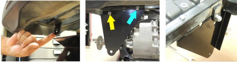
**NOTE:** For matching bolt heads in the bagwell area, a second set of 10mm hardware is included in the BMF lift kit. Repeat steps 10-11 for the passenger side if desired. This will not effect the lift kit.
