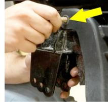
5. Insert a marking device through the thru holes in the shock tower as shown. Mark a drill location on the side of the cross frame.
