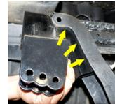
3. Align the hole in the shock tower with the hole in the cross frame as indicated in yellow. If needed, use a screwdriver to align the hole.
