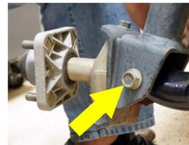
20. Attach the new passenger side steering knuckle to the top of the spindle using (2) 10mm x 80 Hex Head Bolts, (4) 10mm Flat Washers and (2) 10mm Nylock Nuts. Torque the bolts to the correct torque specifications shown on page 2.
