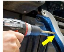
11. Install the shock tower by using the Original Hardware from the upper portion of the shock (yellow arrow) and (1) 10mm x 70 Hex Head Bolt, (2) 10mm Flat Washers and (1) 10mm Nylock Nut (red arrow).
