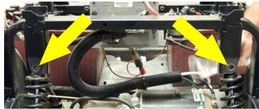
4. Disconnect any wires or cables attached to the motor that could be damaged when lowering the rear suspension.
