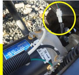
**Safety Note:** The electrical system could be damaged if the cart is NOT in the Tow position and a shock contacts the motor.
