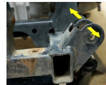
16. Using the Original Hardware, bolt the new BMF A-arm assembly to the chassis in the (4) places where the original A-arms were removed.
