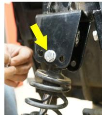
19. Using the Original Hardware, mount the bottom of the shocks to the BMF A-arms. A rubber mallet can be used to align the A-arm in the mounting tabs.
