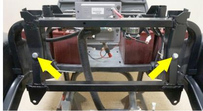
8. Slowly raise the rear axle until the top of the shocks reach the new shock mounts. Install the top of the shocks to the shock mounts using the Original Hardware.
