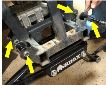
17. Tighten the hardware loosened in Step 14. Keep the A-arm assembly aligned with the frame.
