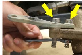
11. Remove the shock assemblies by removing the bolts connecting them to the cross frame and the A-arm. Retain shock assemblies and hardware.
