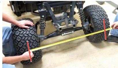
4. Adjust the toe by loosening the jam nut then lengthen or shorten the tie rod by turning the hex shaped rod adjustment. Shortening the tie rods increases the toe-in, lengthening decreases it.
