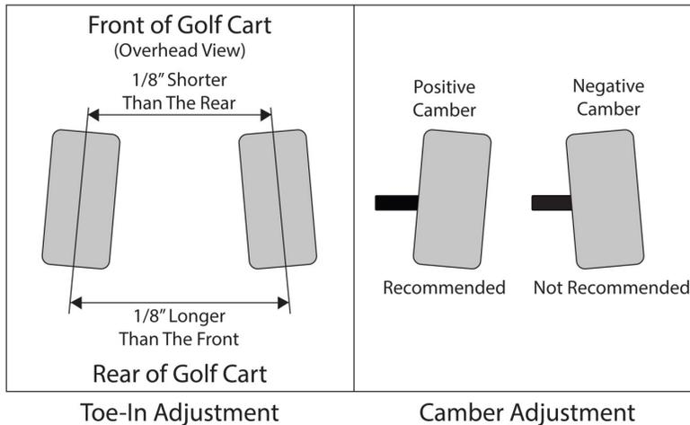
2. Adjust the camber by changing the mounting position of the shock in the shock tower. Mounting the shock to the outside of the cart will make the camber more positive. Mounting it to the inside of the cart will make the camber more negative.
