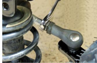
5. Once camber and toe adjustments are finalized and set, tighten all hardware and jam nuts.
