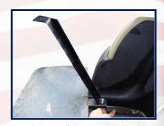
3. Place foot plate on the brackets. Attach bolt on, pointing upward. Attach vertical supports on the protruded bolt and do not secure until next step finishes. Use hardware A-4.
