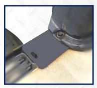
1. Remove all plastic module. Orient holes on mounting brackets with existing holes. Then reattach the plastic module and secure all hardware.
