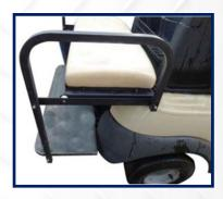
5. Install arm tubes. Use hardware A-1. USE LONGER ONES ON FOOTPLATE SIDE.
