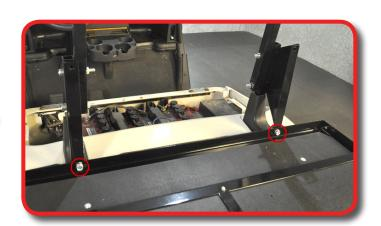
Attach armrests and seat back support using hardware from pack 2 as shown. Be sure to place spacers from hardware pack between the armrest and seat back support bracket. Do not tighten hardware.
