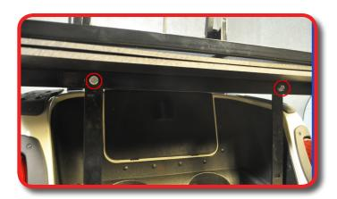
Attach seat frame to brackets using remaining hardware from pack 1 and tighten.
