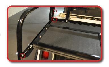
The spacers should be placed as shown on both sides of the cart.
