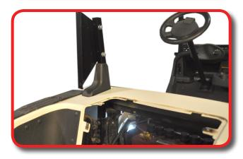
Attach brackets as shown on both sides using hardware retained from step 1
