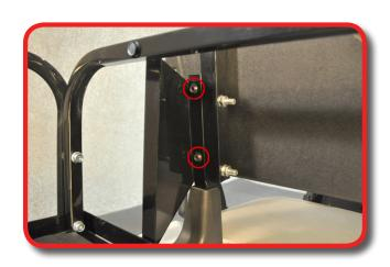
Attach seat back to seat back support using hardware from pack 5. Once this is complete you can tighten down all rear flip seat hardware.
