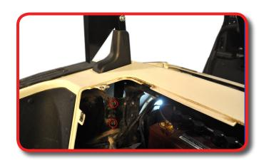
Attach rear struts using retained hardware from rear strut and tighten.
