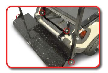
Attach seat back brackets to seat back using hardware from pack 4.
