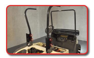
Attach motor cover using hardware retained from step 1.
