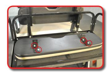
Attach front seat back to brackets using retained hardware from step 1.
