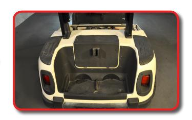
Attach outermost bolts in bagwell and attach bagwell bracket as shown. Be sure the lip of the bagwell bracket faces towards the inside of the cart as shown and tighten.
