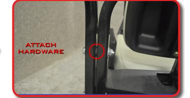
Attach footrest and footrest brackets using hardware from pack 3.
