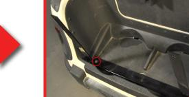
Attach seat frame to bagwell brackets using hardware from pack 1.
