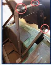
7. Install back support angle / back cushion / back plate (part one installed from step 2-step 4) on cart's main frame using total 6 pieces of existing factory bolts/nuts (include left & right). Picture shows back support angle only.
