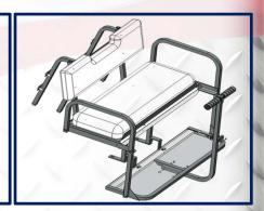
1. First, install the sponge handle onto the grab bar. Separate the clamp and slot the grab bar into the opening. Then attach the clamp onto the grab bar angle, use two 1/4-1 3/4 bolts, four washers and two cap nuts to secure.
