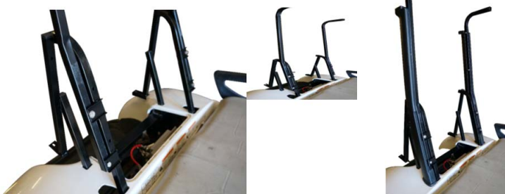
Step 3: Install two rear roof supports on main brackets using hardware D-5
