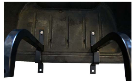
Step 5: Install vertical supports on cart's bagwell area using hardware D-6, install access panel cover back to cart using original factory fasteners.
