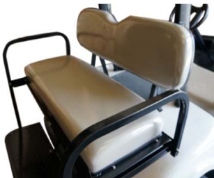
Step 9: Install front backrest cushion using self-tapping screws. Install bottom cushion using (6) self-tapping screws from hardware D-3. install rear seat backrest cushion using hardware D-3 with backrest cushion support bracket.
