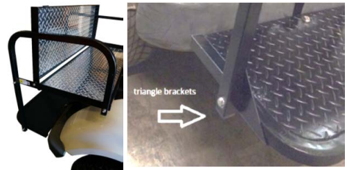
Step 8: Install arm tubes, the bolt points outwards. Use hardware D-1. USE LONGER ONES ON FOOT PLATE SIDE. NOTE: install triangle brackets between armrest and footplate
