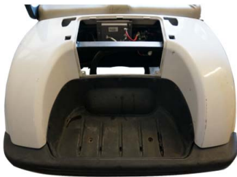
Step 1: Take off canopy / front backrest cushion pad / rear roof support bars (Plastic and steel both) / main brackets (with bag holder and basket) / plastic access panel cover.
