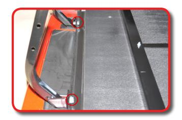
Attach seat frame to bagwell bracket using hardware from pack 1. Ensure that the bottom of the seat frame lies in front of the bagwell bracket as shown.
