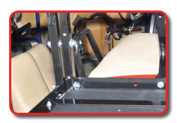
Reinstall front seat backs using hardware retained in step 3.
