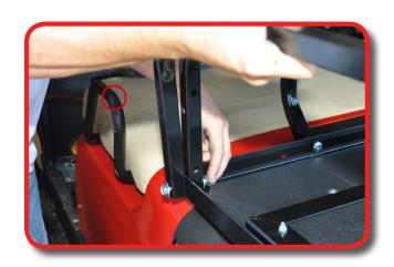
Attach seat back bracket and armrests to seat frame using hardware from pack 2.
