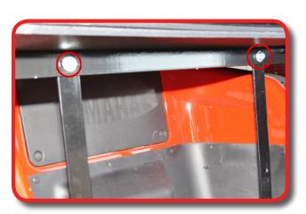
Attach footrest to bagwell bracket using remaining hardware from pack 1.
