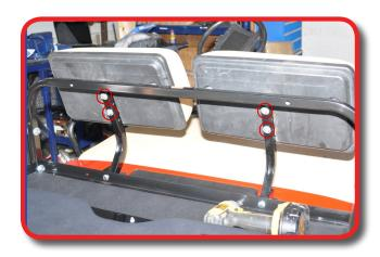
Attach lower location of armrests to footrest using remaining hardware from pack 2.
