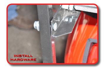
Ensure that when attaching upper bolt through armrest and seat back bracket.
