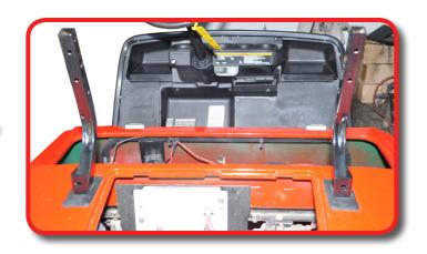
Remove bagwell bolts. Then using a 5/16 drill bit, drill through the vehicle frame where the hardware was removed.
