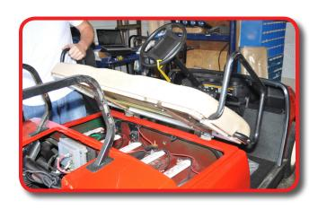
Remove OEM front seat supports. Retain hardware.
