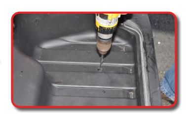
Attach bagwell bracket using hardware from pack 1.
