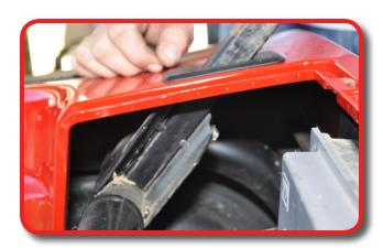
Insert main brackets into holes where OEM front seat supports were removed. Be sure the tabs are pointed to the cart's CENTER, as show. Secure the main brackets with hardware retained in step 6.
