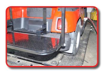
Attach seat back brackets to rear seat back using hardware from pack 3. Tighten hardware.
