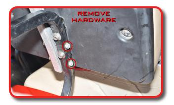
Remove OEM front seat backs. Retain hardware.
