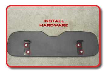
Install rear seat back and rear seat support bracket assembly by attaching end tabs of rear seat support bracket to armrests using remaining hardware from pack 3.
