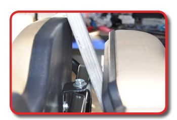
Attach seat bottom and strap to seat frame using hardware from pack 4.
