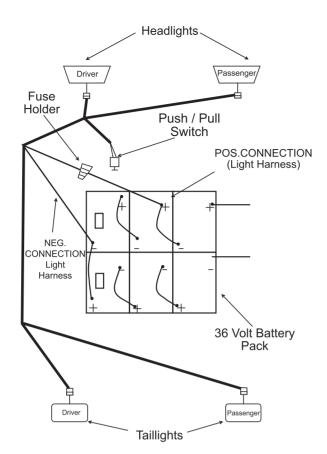
E-Z-Go Basic 36-Volt Wiring Diagram
