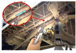
7. Feed the original brake cable, rear end first, into the channel and through the newly drilled hole.
