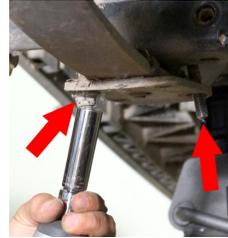
5. Remove the front portion of the leaf spring by removing the bolt on the front shackle. Remove the leaf spring. Retain hardware.
