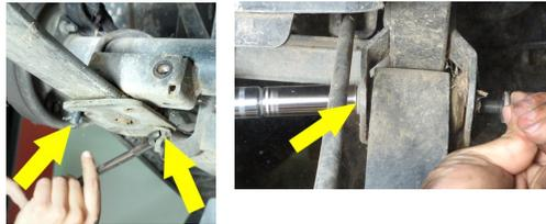
8. Remove the driver side hub by removing the cotter pin and the castle nut. If the hub cannot be removed by hand, use a hub puller, which can be purchased at a local auto store. Retain hardware.
