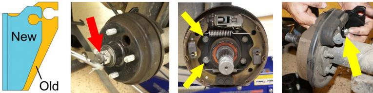
11. Reinstall the hub onto the axle using the Original Castle Nut. Tighten fully. If the cotter pin hole is not entirely visible through the castle nut's gaps, keep tightening. Backing off the nut could strip the hub over time.
