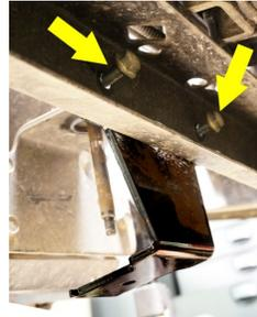
8. Place the Original M10 Bolt through the front engine mount hole. Lower the jack until the bolt threads extend through small hole on the new engine mount bracket.
