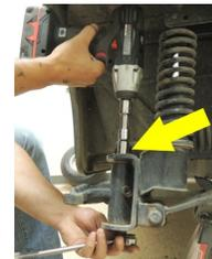
13. Disconnect the shocks from the A-arms and the cross frame by removing the bolts holding them in place. Retain shocks and all hardware.
