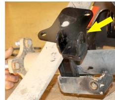
11. Slide the New U-bolt through the shock mounting plate, over the rear axle and through the original leaf spring plate. Tighten the assembly evenly on each side using (2) 10mm Flat Washers and (2) 10mm Lock Nuts. Adjust alignment if necessary.
