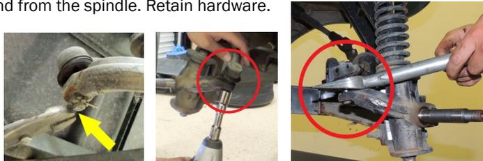
12. Remove the spindles from the shocks as shown in the photo to the right. Discard spindles and retain hardware.
