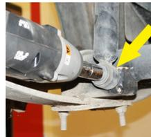
3. With the rear axle supported by the jack, disconnect the leaf spring at the rear shackle. Retain hardware.
