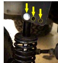
2. Adjust the camber by changing the mounting position of the shock in the shock tower. Mounting the
