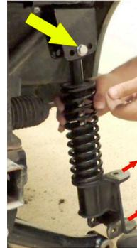
19. Attach the new BMF spindles to the shocks using the Original Hardware from the stock spindles.
