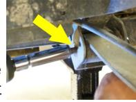
15. Place a riser block on top of the axle and under the leaf spring. When oriented correctly, the wider leg will be towards the front of the cart and the pin on the bottom of the leaf spring will seat into the hole on top of the riser block. Slightly loosening the opposite U-bolt and adjusting the axle position will help with alignment.
