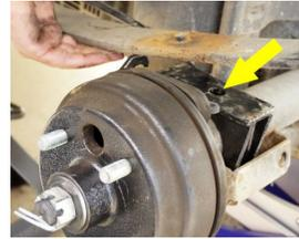
16. Once the spring is seated, identify the new driver side shock mounting plate included in the BMF kit. Place it on top of the leaf spring. The pin will seat in the small center hole. The shock mounting tabs will face towards the center rear of the cart as shown.
