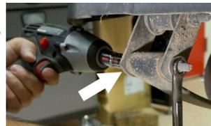
brake cable by loosening the jam nut. Release the driver side brake cable by pushing the tabs inward on the brake cable to allow it to fit through the bracket.
