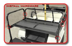
Attach footrest brackets to footrest and armrests using hardware from pack 3.
