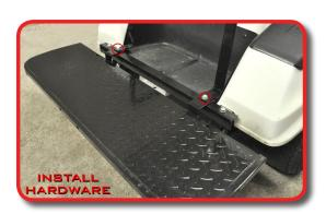
Attach seat frame to the front portion of the main frame brackets using hardware from pack 2.
