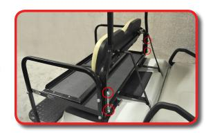
Attach seat bottom and strap to seat frame using hardware from pack 6.
