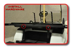
Attach seat back support and armrests using hardware from pack 3.
