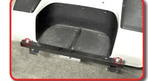
Install main seat frame brackets and front seat lean back brackets to front with retained hardware. Using 8mm hardware from pack 1, mount middle bracket to cart.
