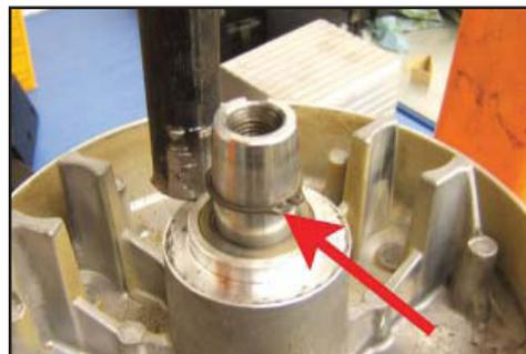
Figure 2 - Snap Ring Removal
