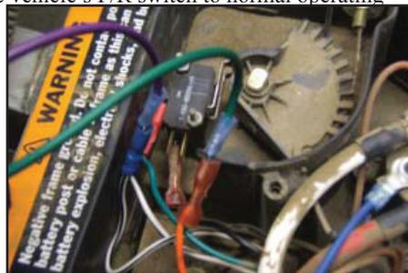
Figure 9 - Relay Wire Connections
