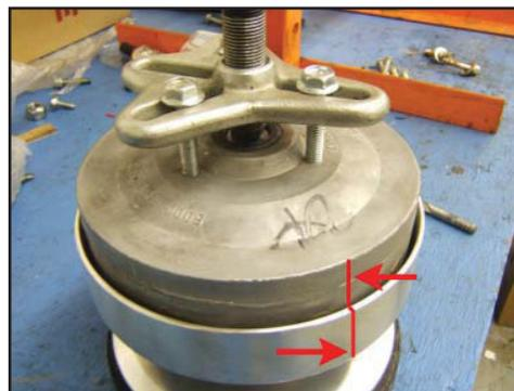
Figure 1 - Clutch Cover Removal
