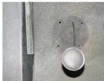
**Step 4:** Place the horn button decal over the horn button. Be sure that the horn button is centered. Mark the four mounting holes using a punch or a marker. Remove the decal and horn button, then drill the 4 marked mounting holes using a 3/16 drill bit. Drill through the floor mat and under body.
