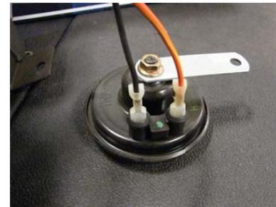
**Step 9:** Mount the horn in a convenient location under the front body of the vehicle.
