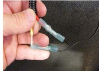
**Step 8:** Connect the black and yellow/orange wires from the headlight bar harness to the horn. Be certain the wires are connected securely.
