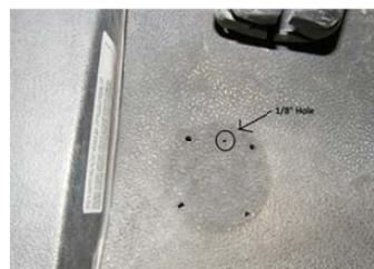
**Step 3:** Thread the horn button's wire lead through the 1/8" hole. Reach behind the floor mat and pull the wire lead under the mat up to the dash area.
