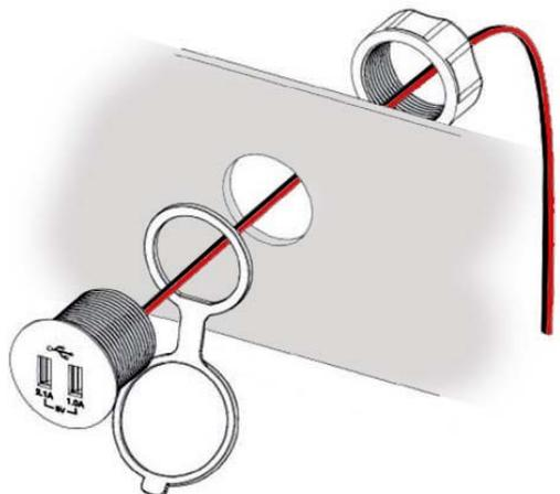
4. Connect the (+) red and (-) black wires to the power source using the wiring diagram below. If using a RHOX Plug & Play Light Kit Harness, connect the wires to the connections used for the 12V outlet. Cut the wires to the desired length if needed.
