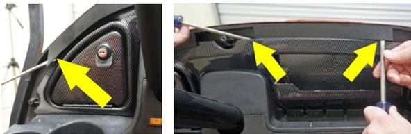
**Step 4:** Insert the 'Christmas Tree' Rivets through the tee holder and into the two pre-drilled holes on the bottom of the dash.
