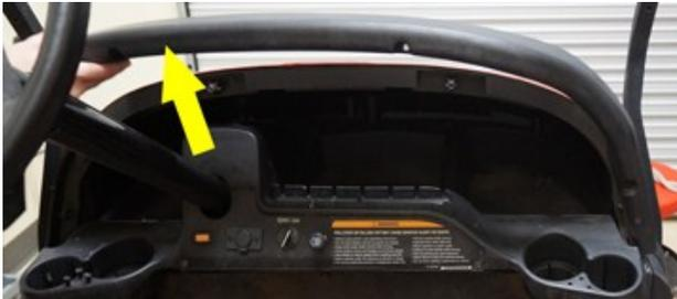
**Step 2:** Insert dash, bottom side first into the space behind the tee holders.
