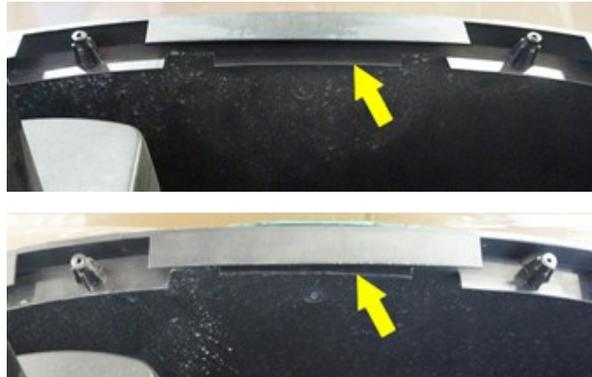
**Step 3:** Starting on one side, pry the plastic that was behind the trim over the top lip of the dash using a flat screwdriver or similar tool.
