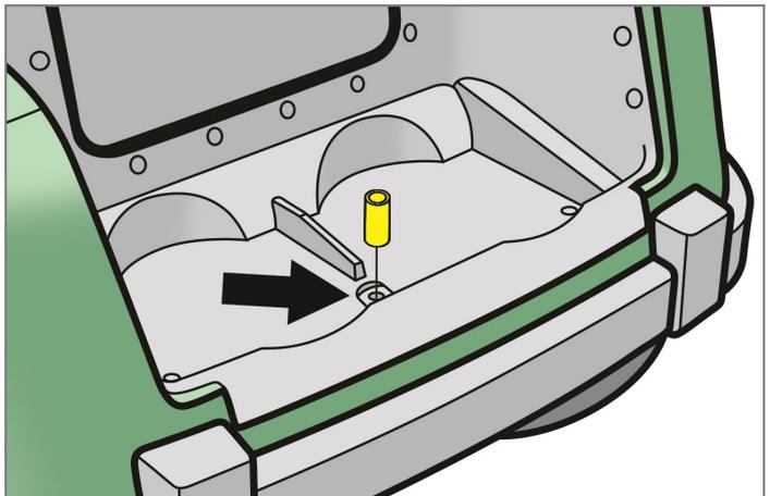
3. Fasten the center of the hitch receiver to the underside of the bagwell area using (1) 12mm x 80mm Hex Head Bolt, (2) 12mm Fender Washers and (1) 12mm Nylock Nut. Hand tighten.
