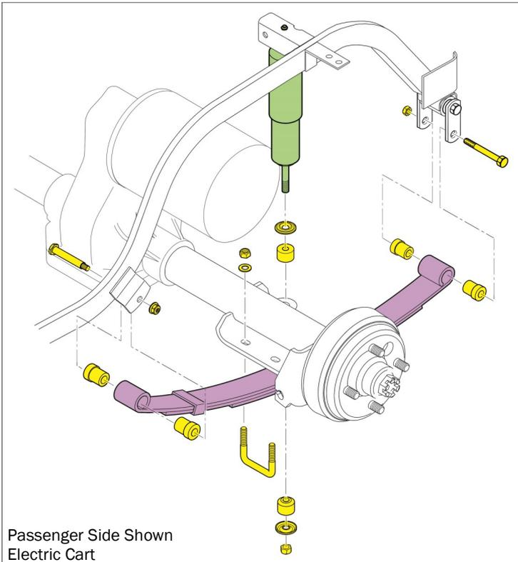
3. Place a lift block (orange) in the perch, on top of the axle.
