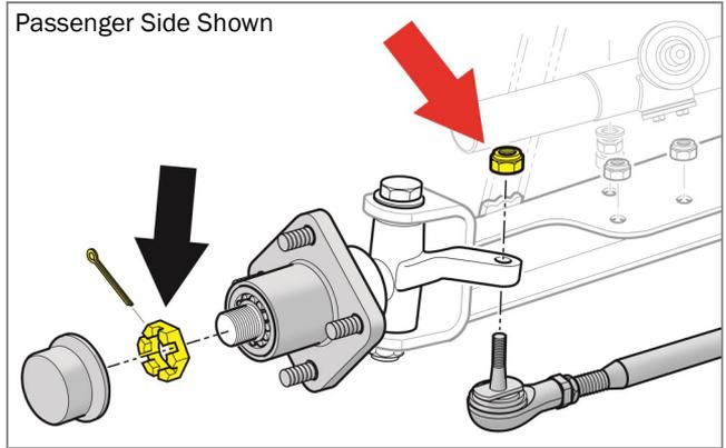
11. Disconnect the steering rack from the front axle (yellow). Retain hardware and spacers. Push the steering rack away from the axle.
