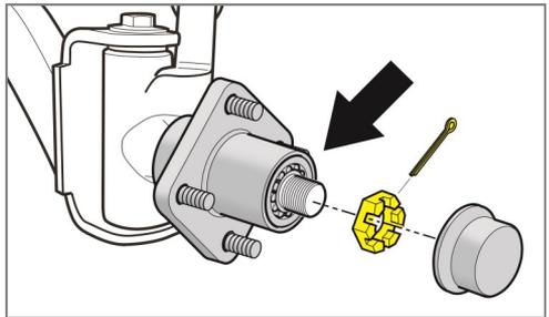
6. Grease the fittings on both spindles using a general purpose automotive grease.
