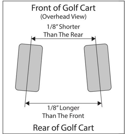
4. Once the toe adjustments are finalized and set, tighten the jam nuts.
