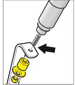
**CAUTION:** Do NOT over torque the hardware. Doing so could break the steering box mounting tabs.
