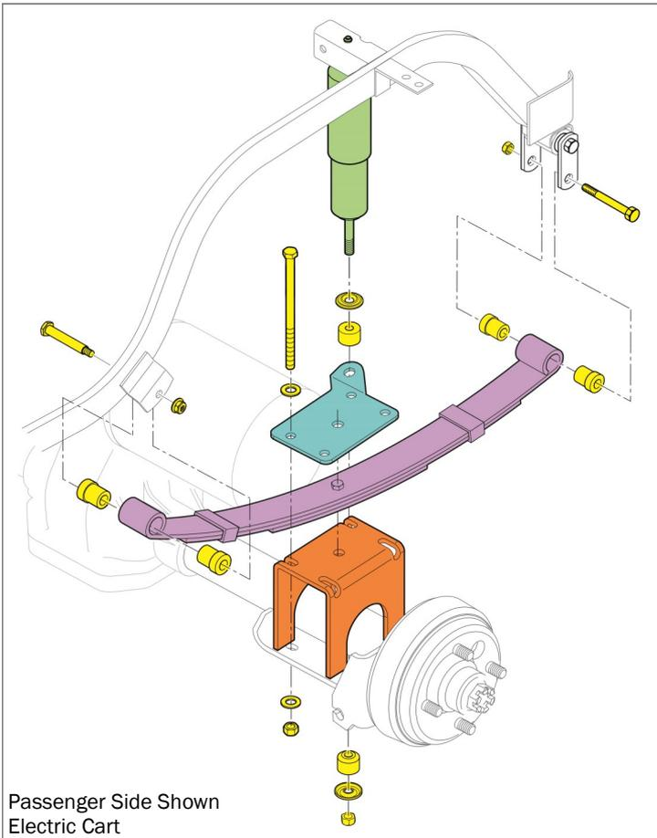
6. Fasten the shock plate, leaf spring and lift block to the perch under the axle with (4) 3/8"-16 x 6-1/4" Shoulder Hex Head Bolts, (8) Flat Washers and (4) Nylock Nuts. Hand tighten bolts evenly on both sides.
