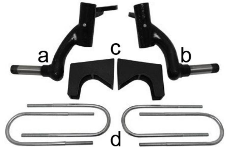
Contents of LIFT-110 E-Z-Go TXT Drop Spindle Lift Kit:
