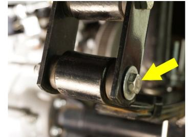
14. Pull down the shocks and bolt them onto the axle brackets using the Original Hardware.
