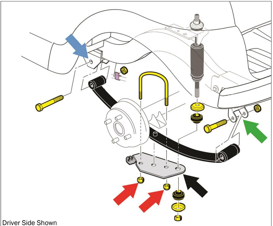
15. Place a lift block on top of the axle, in the perch. When orientated correctly, the lift block will slope downwards toward the front of the cart.
