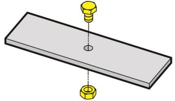
20. Place the centering plate under the lift block perch on the axle as shown on page 8. The 6mm hardware will seat into the alignment hole under the lift perch.
