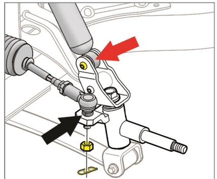
12. Remove the (3) bolts in the steering rack. Retain hardware.
