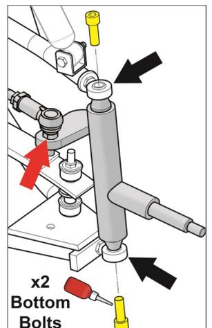
10. Tighten any hardware left loose in this section.
