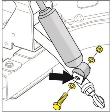
6. Fasten the new front suspension to the chassis where the original suspension was removed using the original leaf spring clamp, (4) 10mm x 45 Hex Head Bolts with Thread Locking Compound and (4) 10mm Flat Washers.
