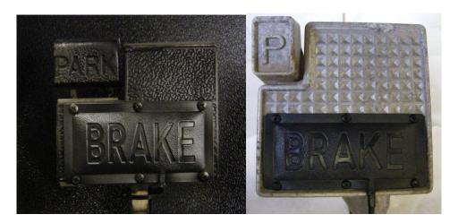
The LGT-138 pressure activated Brake Light Switch is designed to universally mount on the brake pedal of most golf cars. Below you will find our suggestions for mounting the LGT-138 Brake Light Pad. We also suggest purchasing HDW-103 that includes mounting hardware for all applications.
