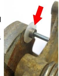
2. Add the step bracket, Flat Washer and Nylock Nut.
