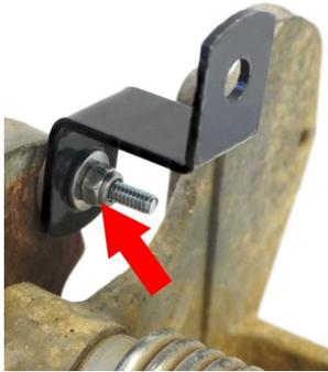
3. Fully tighten the hardware. The bracket will still be able to pivot.
