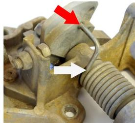
4. Remove and retain the nut from the brake pedal shaft. Do not remove the shaft.
