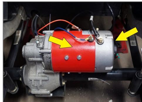
3. Repeat steps 1 and 2 until the 6-10 mile break-in period is complete and the motor is running cooler.
