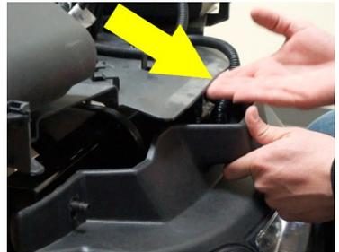
3. Install the headlight bumper using the Original Bumper Hardware. Keep the original nuts and washers in place between the bumper and the shock.
