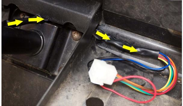
5. Connect the included flasher relay to the turn signal switch wiring harness.
