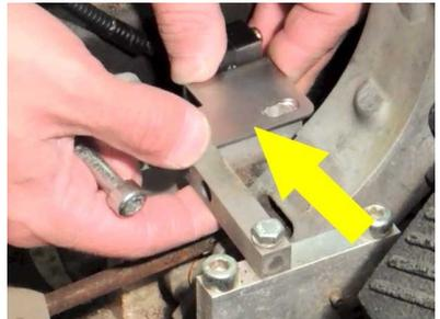
5. Make any adjustments in the brake switch position and tighten all hardware.
