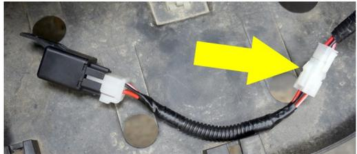
7. Secure the relays and any loose wires out of the way of the cup holders with cable ties.
