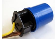
6. If installing the LGT-132A, remove the push-pull switch at the 4-pin connector and replace it with the LGT-590 relay harness.
