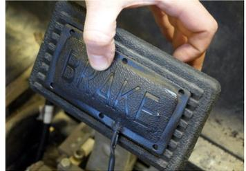
2. If mounting the switch using the Included Screws, fasten the pad directly to the pedal.
