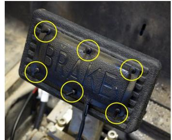
3. Run the brake pad wire around the back of the brake pedal from the passenger side to the driver side of the cart. Make sure it is secured so it will not be pinched.
