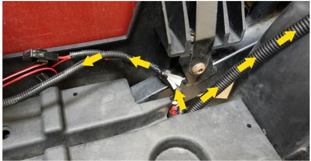
5. Make sure the battery connection leads are able to reach the battery pack. Set the leads to the side. They will be connected after completing the installation of the harness, lights and/or accessories.
