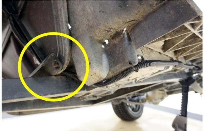
11. Locate the rectangular hole in the bottom of the splash guard. Use a utility knife to enlarge the hole enough to fit the harness.
