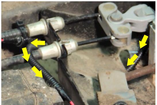
7. Install the LGT-142, time delay, underneath the brake cables using the Included Hardware. There is already a predrilled hole in this location.
