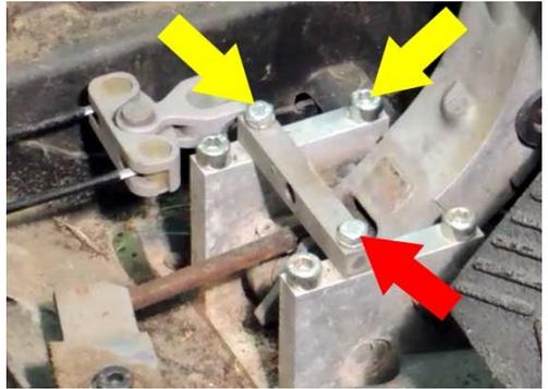
3. Slide the brake switch under the stop bar until the holes align. Reinstall the Original Hardware but do not tighten completely.
