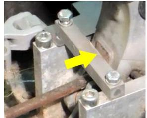
6. Run the brake switch wire through the holes in the pedal compartment so it is next to the brake connector on the deluxe harness.
