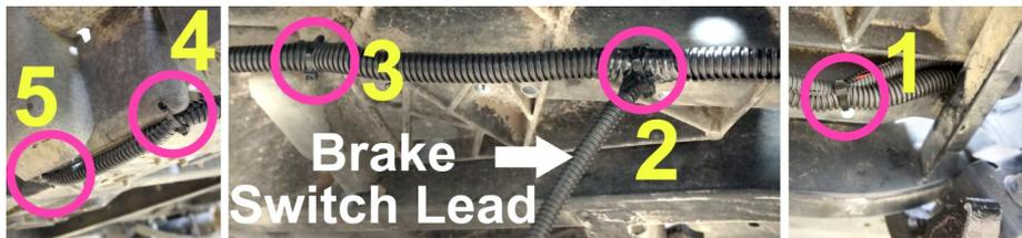
14. Secure the harness away from the steering column with a cable tie.
