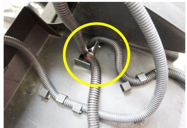
13. Secure the middle portion of the harness to the underbody of the cart. Use a 1/4" drill and drill (5) holes in the plastic underbody.
