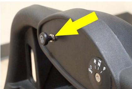
24. Connect the push-pull switch to the 4-pin connector on the harness.
