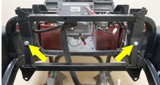
8. Slowly raise the rear axle until the top of the shocks reach the new shock mounts. Install the top of the shocks to the shock mounts using the Original Hardware.
