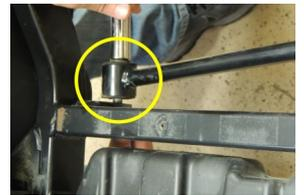
3. Disconnect the top of the rear shocks from the shock mounts. Retain hardware.
