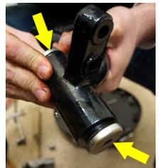
2. Install the new spindles to the bottom portion of the shocks using the Original Hardware. Driver side is shown.
