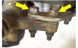
11. Remove the spindles from the lower portion of the shocks by removing the safety pin, nut and bolt. Retain the hardware, thrust covers and spacers. Discard spindles.
