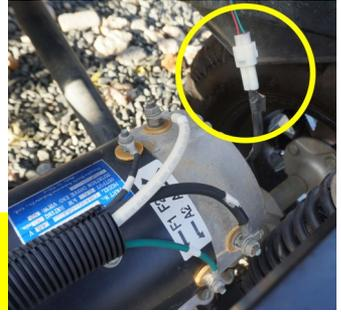
**Safety Note:** The electrical system could be damaged if the cart is NOT in the Tow position and a shock contacts the motor.
