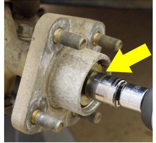
10. Disconnect the steering knuckles from the spindles by removing the safety pins, nuts and bolts. Retain hardware.
