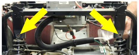
4. Disconnect the 3-pin connector attached to the motor to eliminate damage when lowering the rear suspension.
