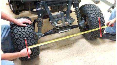
3. Adjust the toe by loosening the jam nut then lengthen or shorten the tie rod by turning the hex shaped rod adjustment. Shortening the tie rods increases the toe-in, lengthening decreases it.
