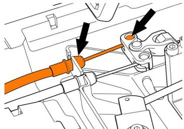
5. Gently pull the driver side brake cable completely out of the cart.
