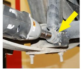
4. Loosen both nuts on the U-bolt then carefully remove the U-bolt. Discard the U-bolt. Retain the leaf spring plate.
