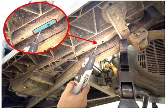
7. Feed the original brake cable, rear end first, into the channel and through the newly drilled hole.
