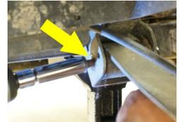
14. Place a riser block on top of the axle and under the leaf spring. When oriented correctly, the wider leg will be towards the front of the cart and the pin on the bottom of the leaf spring will seat into the hole on top of the riser block. Loosen opposite U-bolt and adjust axle position to help with alignment.
