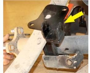
11. Slide the New U-bolt through the shock mounting plate, over the rear axle and through the original leaf spring plate. Tighten the assembly evenly on each side using (2) 10mm Flat Washers and (2) 10mm Lock Nuts. Adjust alignment if necessary.
