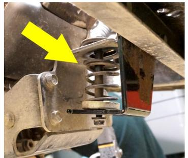
10. After the engine mount bracket is completely installed, remove the jack stands from the rear axle.
