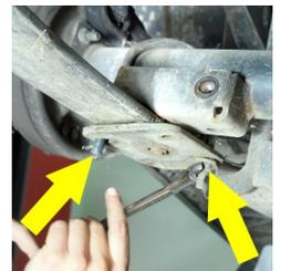
6. Remove the front portion of the leaf spring by removing the bolt on the front shackle. Remove the leaf spring. Retain hardware.
