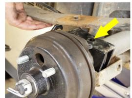
15. Once the spring is seated, identify the new driver side shock mounting plate included in the kit. Place it on top of the leaf spring. The pin will seat in the small center hole. The shock mounting tabs will face towards the center rear of the cart as shown.
