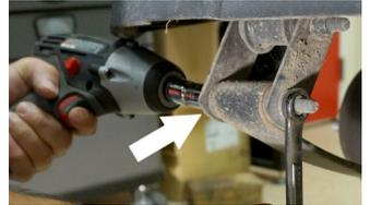
4. Make sure the front wheels are chocked and release the parking brake. Remove and release BOTH brake cables from the rear axle by removing the cotter pins and the pins holding them in place. Release the passenger side brake cable by loosening the jam nut. Release the driver side brake cable by pushing the tabs inward on the brake cable to allow it to fit through the bracket.
