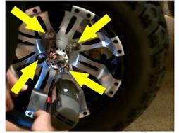
17. Install the (2) rear tires/wheels on the rear hubs.
