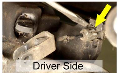
5. Loosen both nuts on the driver side U-bolt then carefully remove the U-bolt. Discard the U-bolt and retain the leaf spring plate.
