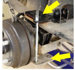
16. Slide the New U-bolt through the shock mounting plate, over the rear axle and through the original leaf spring plate. Tighten the assembly evenly on each side using (2) 10mm Flat Washers and (2) 10mm Lock Nuts. Adjust alignment if necessary.
