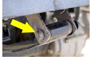
17. Attach the leaf spring to the rear shackle using the Original Hardware. Adjust the axle position if needed for alignment.
