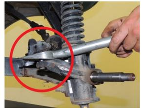
11. Remove the spindles from the shocks. Discard spindles. Retain hardware, kingpin tubes and thrust washers.
