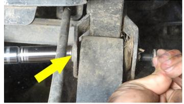
7. Carefully lower the jack to lower the rear axle away from the chassis. Do not remove the jack stands. They support the chassis.
