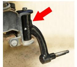
2. Attach the tie-rod ends to the new spindles using the Original Hardware and Safety Pins.
