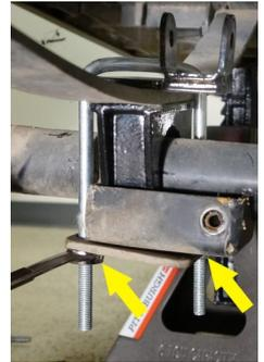
12. Attach the leaf spring to the rear shackle using the Original Hardware. Adjust the axle position if needed for alignment.
