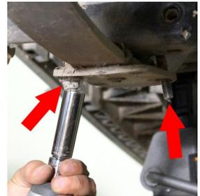
5. Remove the front portion of the leaf spring by removing the bolt on the front shackle. Remove the leaf spring. Retain hardware.
