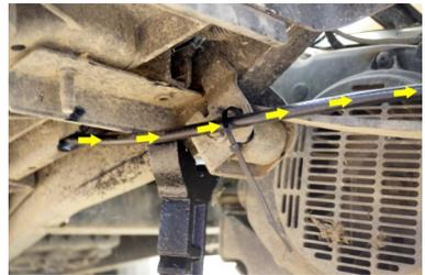
8. Push the front portion of the brake cable through the brake cable bracket and expand the tabs. Reattach the end to the equalizer.
