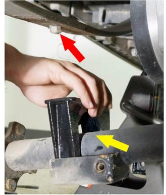
10. Once the spring is seated, identify the new driver side shock mounting plate included in the kit. Place it on top of the leaf spring. The pin will seat in the small hole. The shock mounting tabs will face towards the center rear of the cart as shown.
