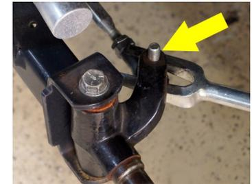
10. Disconnect the steering rack from the front axle. Retain hardware and spacers (shown in green). Push the steering rack away from the axle.
