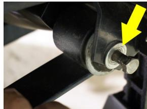
6. Place the leaf spring over top of the axle. Reconnect the leaf spring to the front shackle using the Original Hardware.
